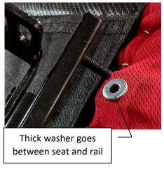
Mount the seat rails as shown above using the hardware included with the rails. You must slide each rail forward or backward to access the respective bolt locations.
