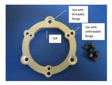
The adapter should be positioned as shown. Attach the wheel to the adapter using the long M4 screws removed earlier through the holes on the rim into the three inner threaded holes in the adapter.
