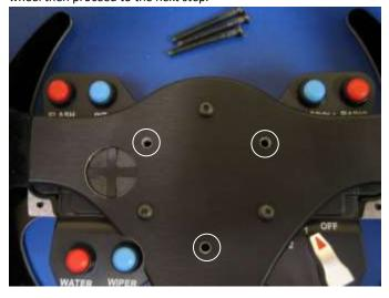
Note the orientation of the mounting adapter shown above. Note the flat at the interior top of the adapter. Be sure to mount in this orientation. There are six outer holes that will align with your 70mm flange. If your flange has threaded holes then mount it with the three short screws at the 4, 8, and 12 o'clock positions. If your flange has unthreaded holes then use the three short screws into the back of the flange at the 2, 6, and 10 o'clock positions. You may use longer M5 screws as needed.
