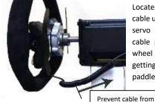
Locate the plug for the USB cable under the tail end of the servo motor. This keeps the cable pulled away from the wheel and prevents it from getting tangled in the shifter paddles.
