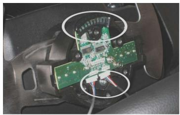
Remove the LED lens piece and unplug the wire harness that go to the wheel buttons.
