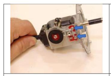
Tighten down the screws that were loosened earlier and then check the shifter for smooth operation.
