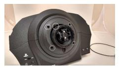
Remove the "nose" cover by first removing the quick-release security screw then removing the four screws securing the nose.
