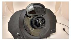
Place the bracket over the front of the servo base and mount using the original screws and the washers supplied.
