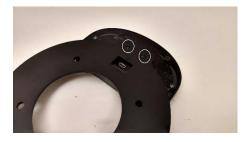
Mount the SRD-R3 to the bracket using the supplied screws into the back of the R3.
