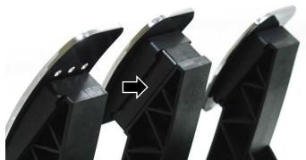
Place the supplied spacer behind the original wedge spacer and reinstall the pedal face with the appropriate length screws provided using the same 2.5mm hex wrench.
