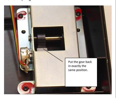
6. Place the pedal back into position and ensure the gear goes back the same way it was.
