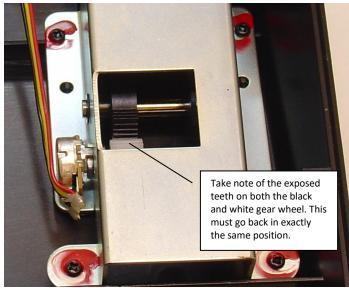
3. Note the number of teeth exposed on the black and white gear wheel. Take a picture if required. The gear must go back in exactly the same position for the pedals to work properly.
