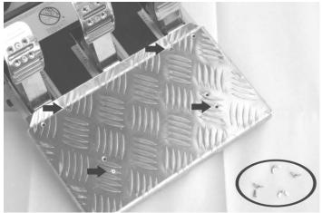
1. Using the 2mm hex wrench, remove the heel plate if your pedals are set up for "F1 Style" arrangement. There should be 4 screws securing the plate as indicated above, there may be extra holes which are left empty. There may be wing nuts securing them from underneath. Place the hardware in a bag and label the bag "heel plate". Set the heel plate and the bag aside.
