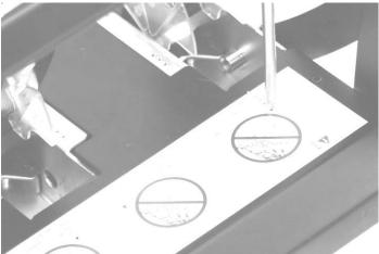
3. Remove the 4 black screws concealed by the warning label. Feel for them with your finger and dig them out with the tip of the screwdriver. Place the screws in another bag and mark it "top screws."
