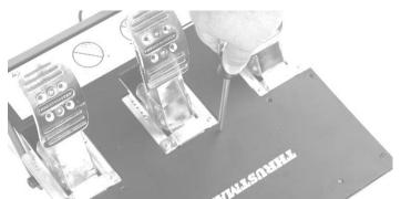
4. Remove 10 more exposed screws at the top of the cover plate and add those to the bag marked "top screws." The cover should now lift off, lift the front first and then 'unhook' the cover from the back. Set the cover and bags of screws aside.
