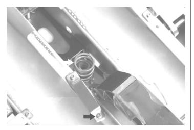
6. Swing the pedal forward and remove the spring (white arrow) with the gas pedal spring. Smear some grease from the original spring onto the new spring.
