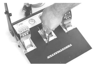
9. Place the top cover over the pedals, hooking it at the back first. The center pedal may have shifted to the side and may need to be centered in the opening to align correctly. Make sure all the wires are in their correct positions so they do not get pinched. Some of the glue originally used may have come undone. Re-install the 14 screws on the top of the cover plate. Then re-install the 6 screws to the back of the plate.
