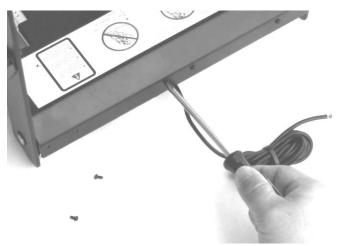
2. Remove the 6 black screws at the back of the pedal assembly. Place the screws in another bag and mark them "back screws." Set them aside.
