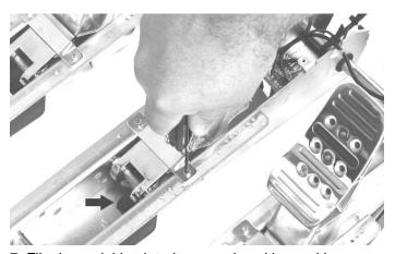
7. Flip the pedal back to its normal position making sure the potentiometer engages the pedal exactly as it was (black arrow). Compare this to the untouched clutch pedal and be sure they are the same. Secure the pedal hold down plate using the original screws.
