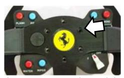
Remove the 3 or 6 screws securing the original wheel to the hub.
