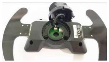
Plug the quick-release into the plug of the internal circuit board and place the quick-release into the rear housing.
