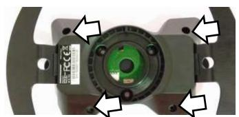
Remove the 4 screws to open the back cover.
