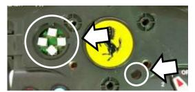
Temporarily remove the D-Pad and grounding spring.
