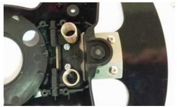
Insert the pre-assembled paddle into the slot and secure to the original plastic pivot with the 2 original screws. Repeat the last 3 steps on the other side.
