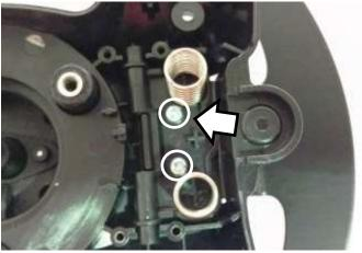
Temporarily set aside the paddle springs. Then remove the 2 screws securing the paddles to the pivots.
