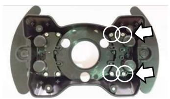
Starting with one side first, remove the 4 screws holding the paddle springs in place.
