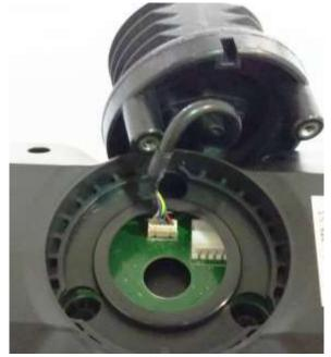
Remove the Quick-Release and unplug the internal cable.
