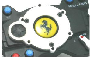
Mount the adapter ring to the wheel hub using the 3 socket head screws provided.
