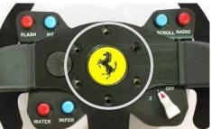
Remove the 3 or 6 screws securing the original wheel to the hub.
