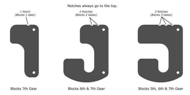
To insert the gate blocker you must loosen the screws on the left side of the gate plate, remove the screws on the right side of the gate plate, slide the gate blocker into place then replace the screws and tighten all four screws.
