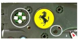
Carefully reposition the D-Pad and grounding spring if they have become dislodged.
