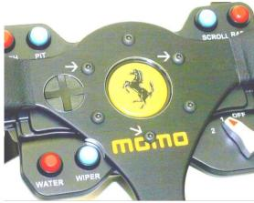
Mount your steering wheel with the 3 LONG screws where indicated by the arrows. If your original wheel had six screws then use the SHORT screws provided in the remaining holes.
