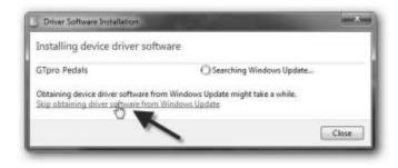
Windows will install its internal drivers. The pedals are powered from the USB port, no external power is required. You should see the LED pulse a red "heartbeat" signal.
