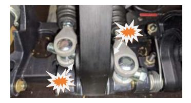
When placing the bushings on the slave cylinder, it does not matter in which position they are placed, the resulting firmness is the same. Use the table below to achieve the desired firmness, where 1 is the softest combination and 10 is the firmest combination.
