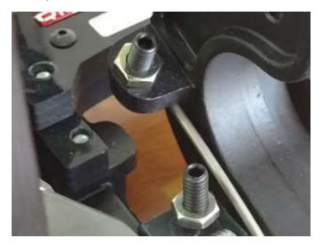
Similarly, the clutch pedal ending position can be adjusted by turning the stop screw located to the right of the pedal. Turning the screw clockwise will reduce the travel, while turning the screw counter-clockwise will increase the travel. Tighten the jam nut when the adjustments are complete to prevent the setting from changing.
