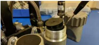
Remove the "leak-prevention" stoppers from the reservoir
