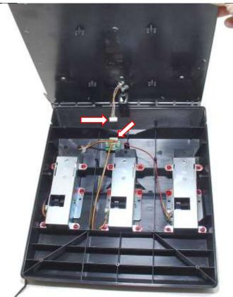
Carefully lift the cover from the near end with one hand and reach in with the other hand to disconnect the 6-pin plug from the circuit board. Do not lift the cover abruptly as this may cause damage to the connector.
