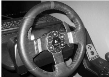
Remove these 6 screws from the original wheel using a 5mm hex key.
