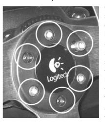
over the hub. Be sure the plate seats centered over the hub and no wires are pinched. Using 2 of the 6 original screws, install into the top and bottom holes and align the wheel into position. Tighten them down and be sure the wheel seats evenly
