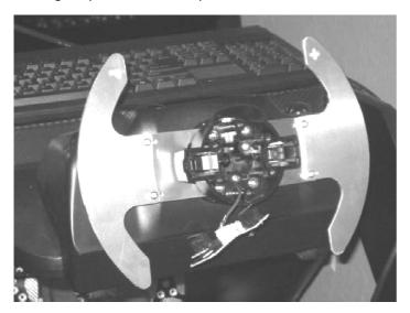
Mount the paddles to your liking using the 4 screws provided. The paddles may be mounted to the front or the back of the paddle brackets, depending on your preference. To install the paddles from behind, rotate the wheel 90 degrees and install the screws from the back side.
