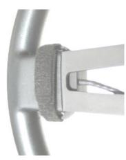
Secure the Push-to-Talk box to the wheel spoke as shown by threading the Velcro strap through the eyelets and then folding them onto themselves so they lock together.
