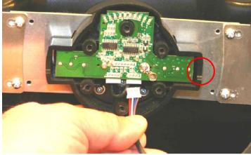
Plug the button box into one of the two connector
