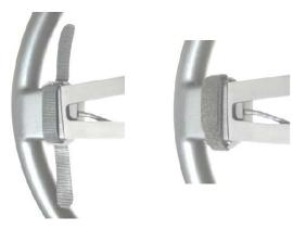
Secure the button box to the wheel spoke as shown by threading the Velcro strap through the eyelets and then folding them onto themselves so they lock together.
